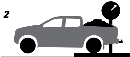
2 Load placed over the rear half of the vehicle determines rear spring selection Ensure total weight does not exceed manufacturers axle load limit
