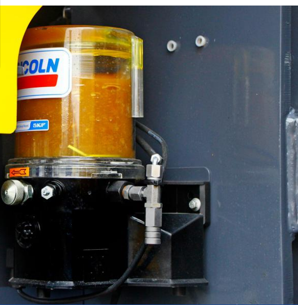
Auto lubricating to minimise daily maintenance
