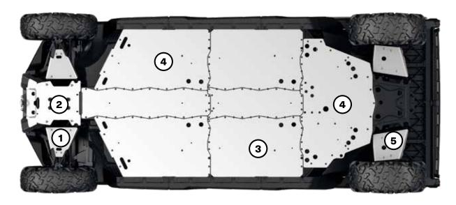
For ultimate durability and strength, all our Aluminum Skid Plates are made with High Strength 5052 H32 Aluminum 3/6" (4.5 mm) thick.
