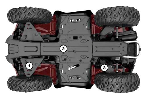
Our plastic plates glide smoothly and silently over obstacles, offering great protection in rough terrain. Made of ¼" (6 mm) thick abrasion-resistant thermoformed High Molecular Weight Polyethylene (HMWPE).
