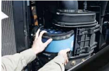
The air filter is easy to remove and the dust is aspirated and ejected in the exhaust
