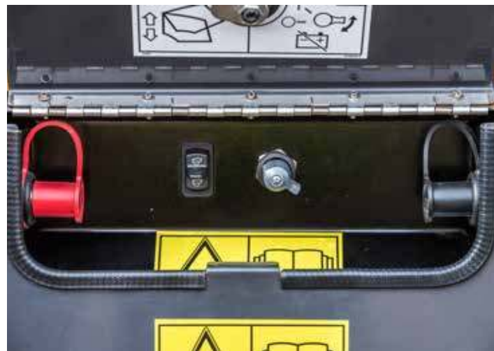
Hood opening and battery on/off switches. In case of flat battery, hood can be opened externally with Remote jump start
