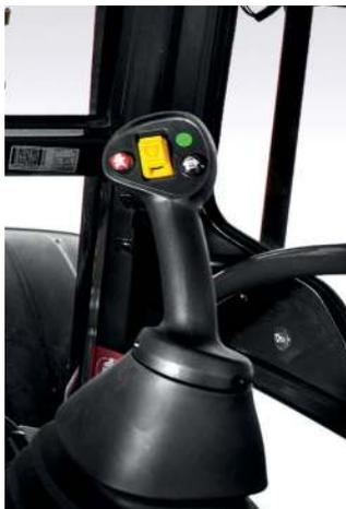
A single control joystick for all the loader functions
