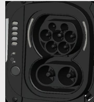
The new 500e is equipped with a CCS\* COMBO 2 Smart Charging Port that enables both public AC and DC charging as well as simple domestic AC charging. The port is positioned in the right rear side of the vehicle and gives immediate feedback on the charging status as well as possibility to manage set charging schedule or immediate charging.
