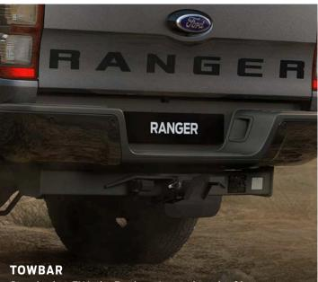
Standard on FX4, the Ford-engineered tow bar<sup>3</sup> has a 3.5 tonne capacity and is fully integrated with the chassis.
