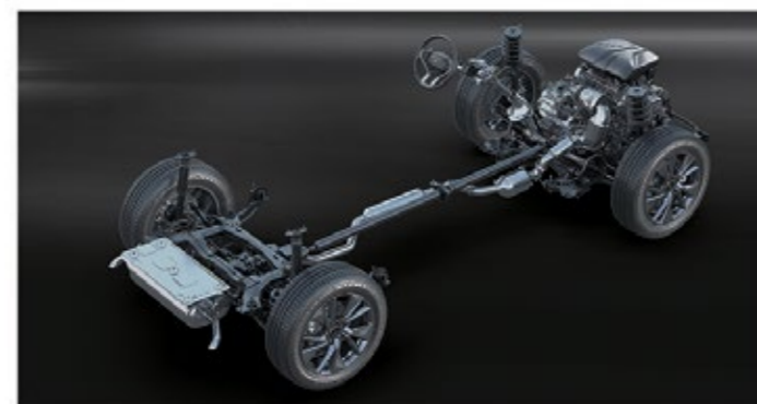
Front Macpherson Rear Multi-link Independent Suspension + AWD
