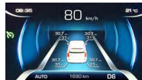
The Haval H9 is also fitted with an active **Tyre Pressure Monitoring System (TPMS)**. Safety experts believe that incorrect tyre pressures contribute to around 80% of accidents involving punctures, which is why tyre pressure monitoring systems are now mandatory in the US. The H9 TPMS keeps an eagle eye on tyre pressures and alerts you to any abnormality. As well as being a great safety feature, driving with the correct tyre pressures also delivers a smoother ride and better fuel efficiency.
