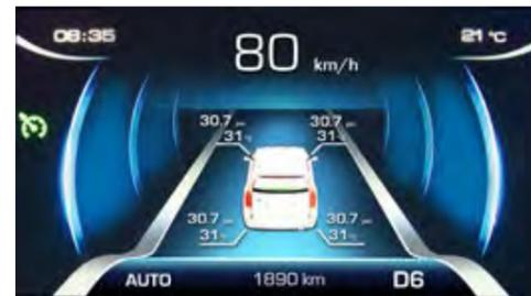
The Haval H9 is also fitted with an active **Tyre Pressure Monitoring System (TPMS)**. Safety experts believe that incorrect tyre pressures contribute to around 80% of accidents involving punctures, which is why tyre pressure monitoring systems are now mandatory in the US. The H9 TPMS keeps an eagle eye on tyre pressures and alerts you to any abnormality. As well as being a great safety feature, driving with the correct tyre pressures also delivers a smoother ride and better fuel efficiency.
