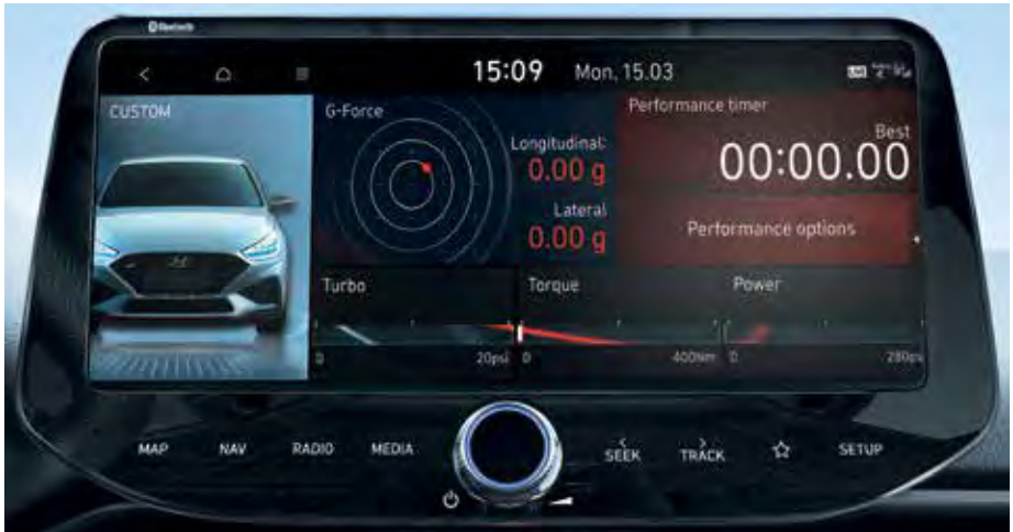
The Performance Driving Data System lets you monitor and improve your driving performance with updated graphics for even more ease of use. See: power, torque, turbo boost, G-force as well as a lap and acceleration timer.
