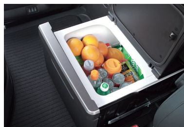
Cooler and warmer drawer (Refrigerant and electric coil method)
