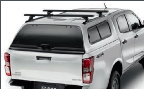
Canopy Roof Bars (Available for Crew Cab Ute models. Sets for 80kg* or 150kg* available.)
