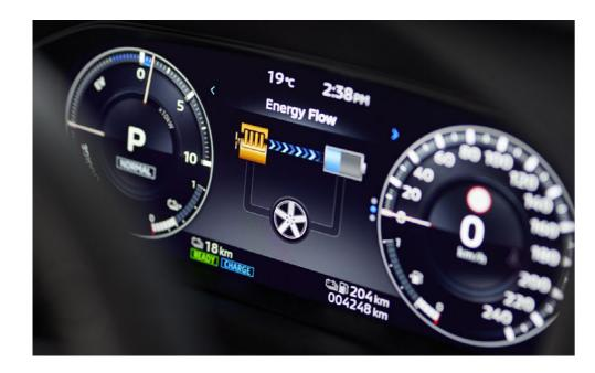
At the heart of the **Outlander PHEV** energy system is technology that seamlessly merges the silent twin electric motors with the 2.4 litre MIVEC petrol engine. Directly in front of you the 12.3-inch Digital Driver Display screen will show you the car's energy flow and drive modes.
