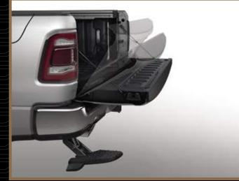
**STEEL DEPLOYABLE BED STEP** eases cargo access. It's foot-controlled for use or to tuck it back under the bed and features a slip-resistant rubber coating.
