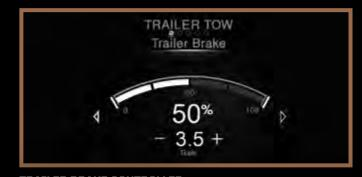
**TRAILER BRAKE CONTROLLER** It's just part of dozens of menu options in your control. This shows the brake set at 50% of operation with a 3.5% gain.
