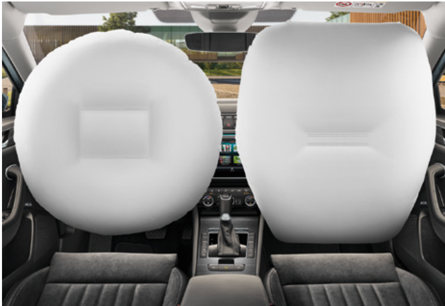
FRONT DRIVER AND PASSENGER AIRBAG While the driver airbag is enclosed in the steering wheel, the passenger airbag is located in the dashboard.
