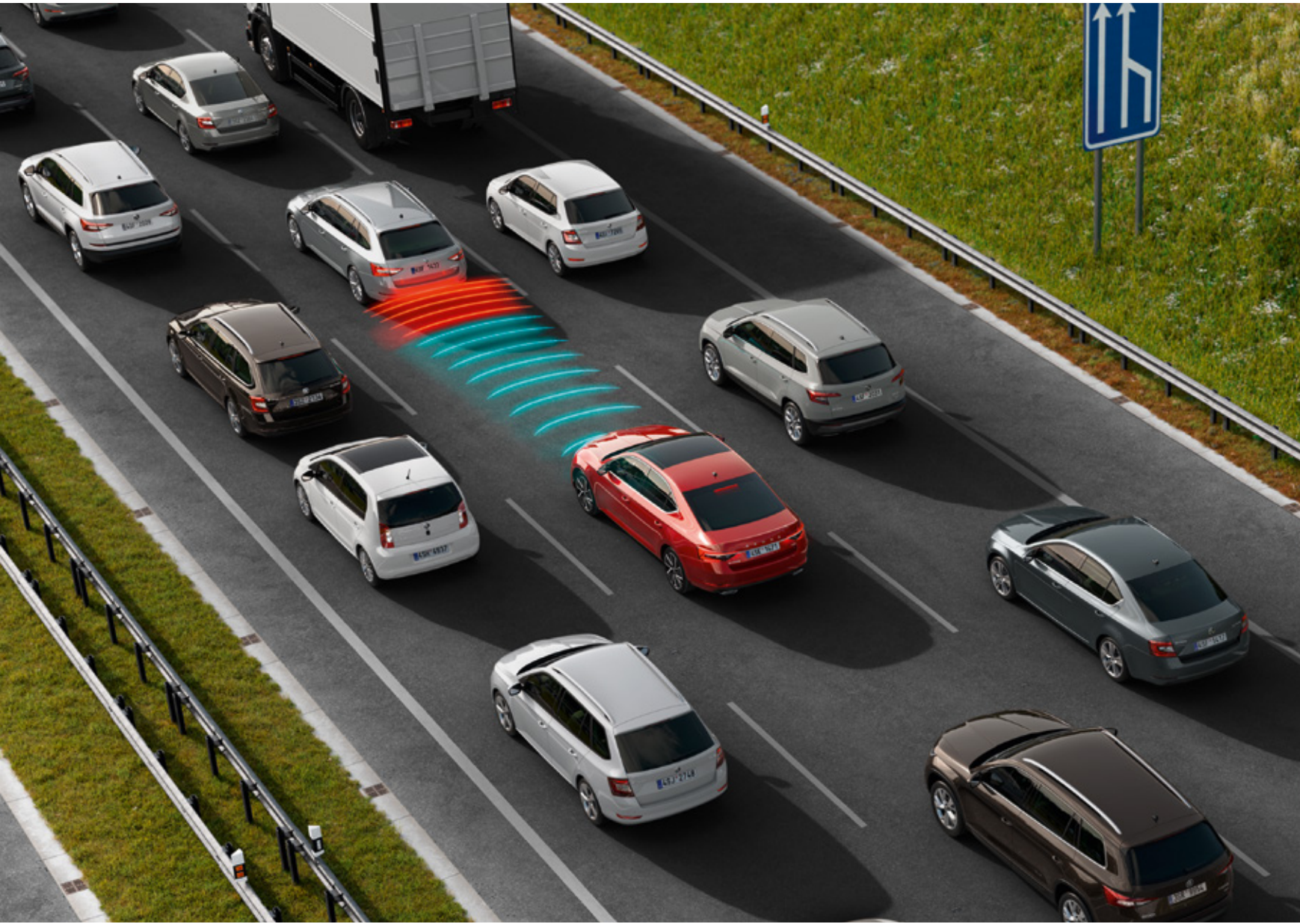
TRAFFIC JAM ASSIST o This function is designed to facilitate driving in traffic jams. By controlling the engine brakes, and steering, it makes the vehicle pull away, brake, and turn to copy the movement of the surrounding vehicles (at speeds of up to 60 km/h). If lanes are not detected at speeds of up to 30 km/h, or only one lane (line) is detected at speeds of up to 60 km/h, the Follow Drive system follows the trajectory of the vehicle in front of you until lane markings are available again.
