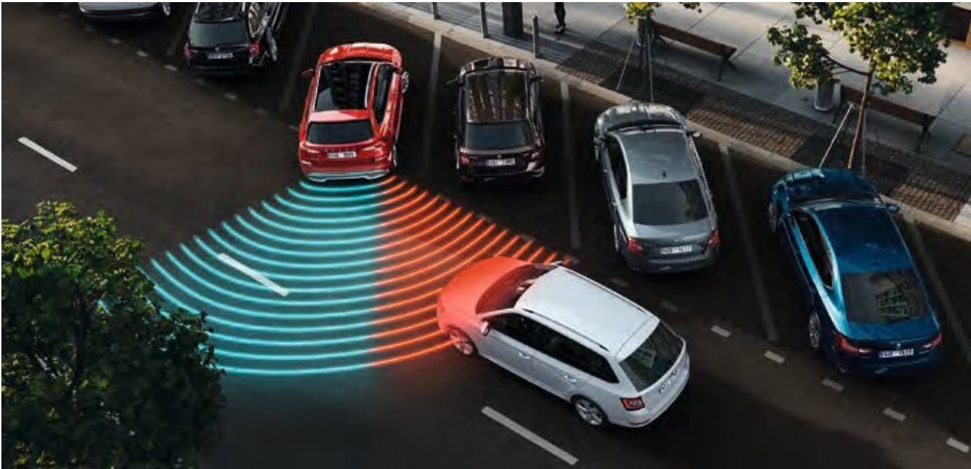
REAR TRAFFIC ALERT This assistant, which comes as part of the Side Assist system, helps you reverse safely from a parking space during poor visibility. It can even engage the brakes automatically if it detects imminent danger.
