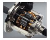
On muddy or snowy surfaces, one wheel may slip or be lifted into the air. In this case, the locking differential forces both wheels on an axel to turn in unison, allowing the vehicle to recover its traction.
