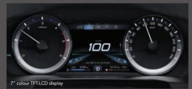
TRIPLE-MODE DIGITAL SPEEDOMETER DISPLAY
