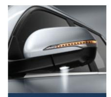
Side repeater and puddle lamp mounted on the back of the outside mirror
