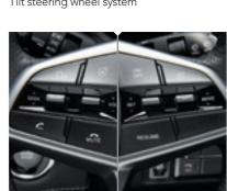
Remote control switches and cruise control system on the steering wheel
