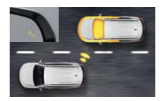
Lane Change Assist (LCA) Detects vehicles rapidly approaching from behind and flashes a warning light on the
