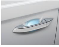
2-channel touch sensing door handle. Outside door handle lamps
