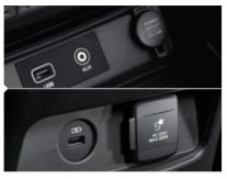
USB port and power outlet on centre console, Smart key USB port and 220V/115V inverter in 2<sup>nd</sup> row
