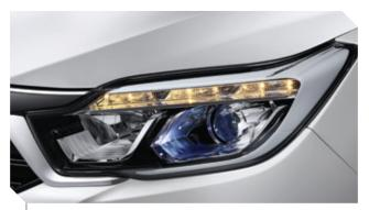
Elegant front light cluster with high-intensity-discharge headlamps for excellent night vision; LED daytime running lights, positioning lamps and directional indicators
