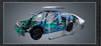
The SGP and ring-shaped passenger safety cell absorb and direct impact force around the cabin, rather than through it.
