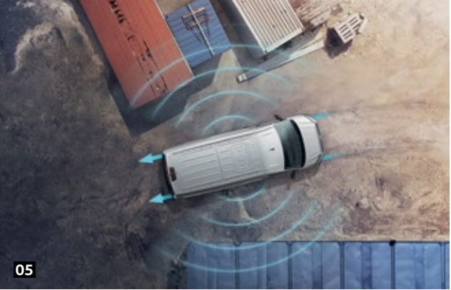
05 Sensor-Based Side Protection*. Monitors the vehicle sides and emits visual and audible warnings if coming hazardingly close to pillars, walls or pedestrians. | KS | KA |
