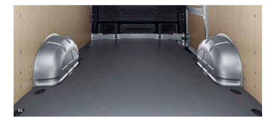
01 Wooden floor. 1), 2) This 10 mm thick wooden floor for the load compartment provides the optimum surface for your cargo to rest on. The robust beechwood ensures excellent stability and durability. | KA |
