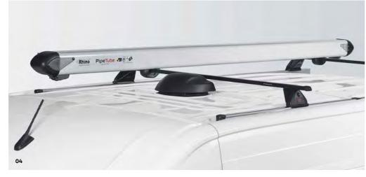
03 Roof bars. The carrier is made of aluminium and galvanised sheet metal and attached to the C rails. It is only available for the normal roof variant and can hold up to 150 kg. | KA | PL |
