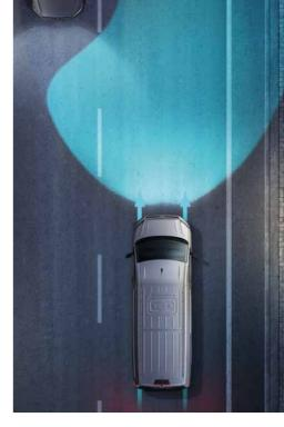
= A High beam assistant "Light Assist". Automatically dips the headlights for oncoming vehicles or vehicles travelling ahead before they are dazzled. When activated, the system automatically switches on the main beam headlights when the vehicle is travelling above 60 km/h in complete darkness. KA PL PR KP FG
