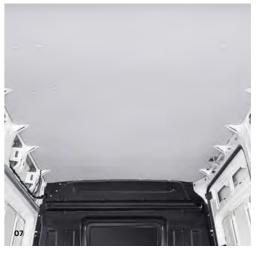
07 "Vario Protect" headliner. The contoured head- 08 Shock absorbing rear step. Mounted on leaf liner features an especially robust design to protect springs, the step can withstand light collisions. the roof. The "Vario Protect" headliner is resistant | KA | PL | PR | FG | to impacts, chemicals and environmental influences.
