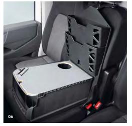
06 Multifunction box for the front passenger bench seat. With a variety of storage compartments and a cover which can also be used as a writing surface, this box can expand the cockpit into a mobile office. The removable box is secured between the driver and front passenger using the seat belt and a fastening on the head restraint. | KA | PL | PR | FG |
