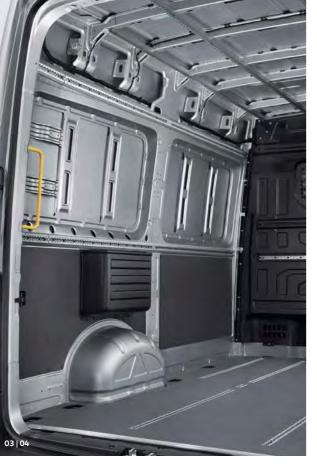
**03** Storage boxes above the wheel housings. They are fitted above both wheel housings in the load compartment and provide space for lashing straps, tools, high visibility vests and gloves. | KA | PL |
