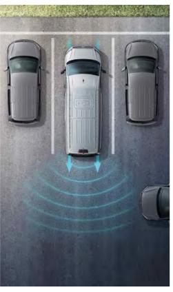
Blind Spot Monitor and Rear Traffic Alert.1) Emits an audible warning when reversing out of a parking space and another vehicle is getting too close. If the driver fails to react, the system can minimise the consequences of a possible accident and, in the best case scenario, prevent an accident entirely, by applying the brakes. | KA | PL |
