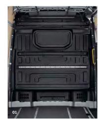
01 Partition without window. The partition wall according to DIN 75410-3 is completely closed. A roof compartment above the driver's cab is available as an option for the high roof variant and is a standard feature for the super high roof variant. | KA |
