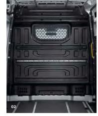
02 Partition with window and safety **guard.** The angled window prevents reflections from impairing the driver's field of vision. The guard provides protection for the window, driver and passengers, for example during abrupt braking manoeuvres. Two window variants are available: a closed partition window or a flexible sliding window. | KA |
