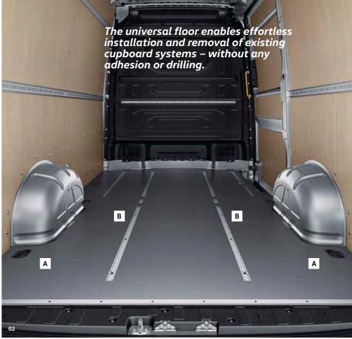
**02** Universal floor.<sup>1), 2)</sup> This wooden floor is the ideal basis for retrofitting shelving and cupboard systems available from a range of manufacturers. Special adapters (A) enable cupboard systems to be easily attached using the notches. The lashing rails (B) are either available as longitudinal or transverse rails. | KA|
