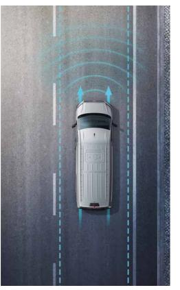
Countersteers if a lane is left unintentionally while alerting the driver at the same time by using a warning tone and information in the multifunction display. | KA | PL | PR | KP | FG |
