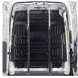
**02** Two clamping bars. Enable you to safely transport a variety of different cargoes. The clamping bars can be quickly inserted and removed for flexible positioning in the load compartment. | KA | PL |
