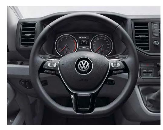
01 Heated leather-covered multifunction steering wheel. It gives you good grip and is extremely user friendly. The radio or navigation system, a mobile phone, and the cruise control system can all be controlled using its buttons. | KA | PL | PR | KP | FG |
