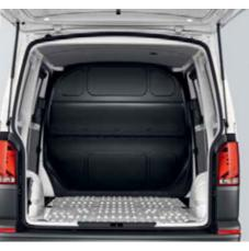
08 Loading sill protection (rear bumper.<sup>7)</sup> Protects the painted rear bumper from scratches when loading and unloading. The plastic trim is available in Silver or Black. | KA | KO | KP |
