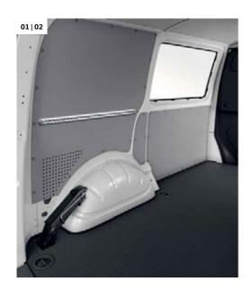
01 High side panel trim (hardboard).<sup>1)</sup> Full-height protection of the side panels from the floor to the roof frame. |KA | KO | KP |
