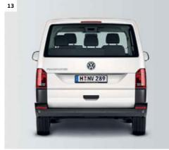
12 Tailgate without window. Allows convenient loading and unloading with a large opening height of max. 2,200 mm<sup>8)</sup>. |KA | KP |
