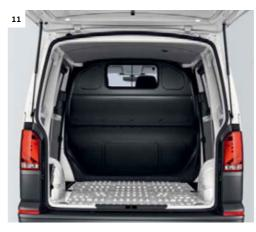
10 Partition, high with window. The window is made of safety glass. | KA | KO |
