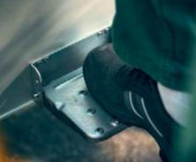
Saves a lot of energy. The step made of stainless and anti-slip aluminium checker plate facilitates access o the load pl
