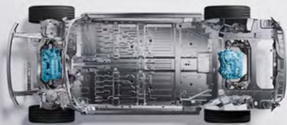
Front Double Wishbone + Independent Rear Five-link Suspension
