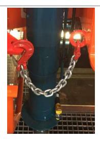
Illustration 13-00 10; Example stabilizer outrigger locking mechanism
