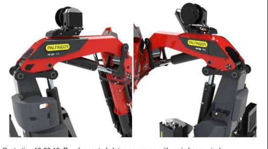
Illustration 10-00 10; Powder-coated plates on cranes with main boom winch
