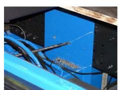
▶ Drill the holes in the console plates.
