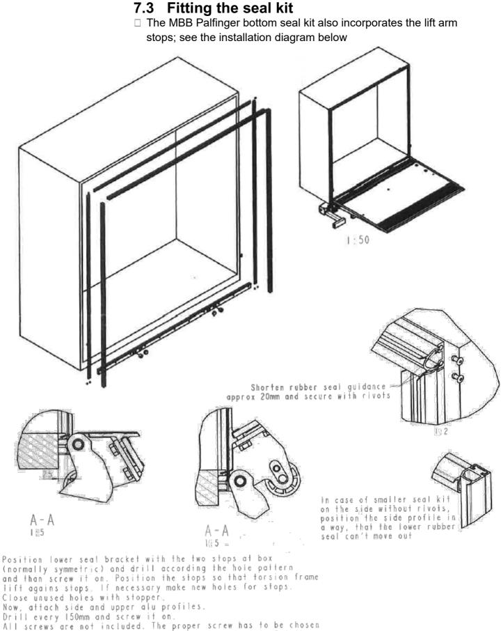
All screws are not included. The proper screw has to be chosen by the body builder in accordance with his material. Cut the rubber to your desired length. Secure them with rivots.
