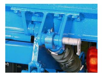
• Grease the pin and bolt the tilt cylinder to the platform.
