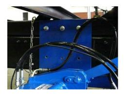
Bolt the console plates to the vehicle chassis. In the process, note the tightening torques in the general installation diagram and in the following table.
