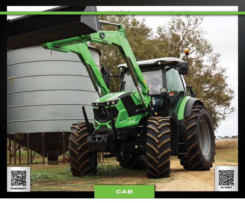
The Deutz-Fahr 6G Series of tractors were completely designed from the ground up by the German engineering team. The design brief was to create a tractor for Australian conditions to be built in Germany. The combination of a six cylinder Deutz engine matched with the highly efficient German ZF transmission and class beating hydraulics creates the 6G PowerVision.
