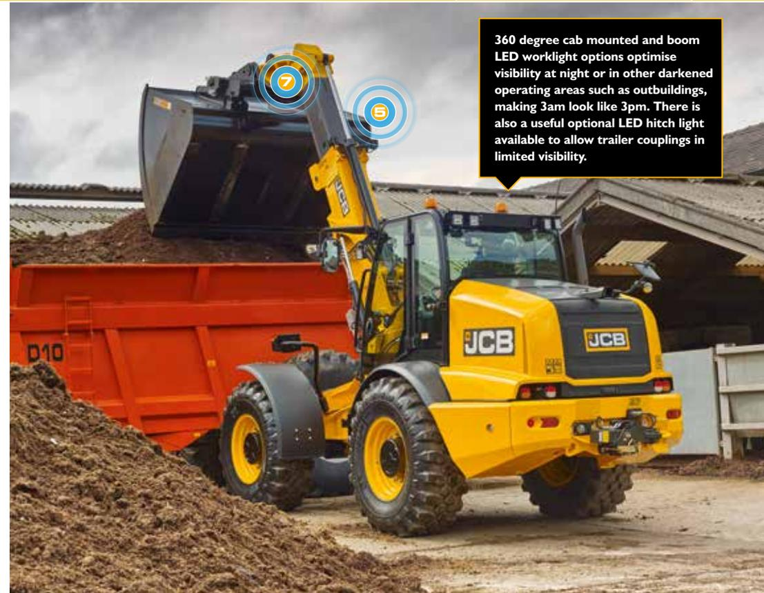
360 degree cab mounted and boom LED worklight options optimise visibility at night or in other darkened operating areas such as outbuildings, making 3am look like 3pm. There is also a useful optional LED hitch light available to allow trailer couplings in limited visibility.
