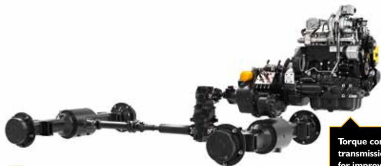
Torque converter locking on the transmission gives 100% efficiency for improved fuel economy.
