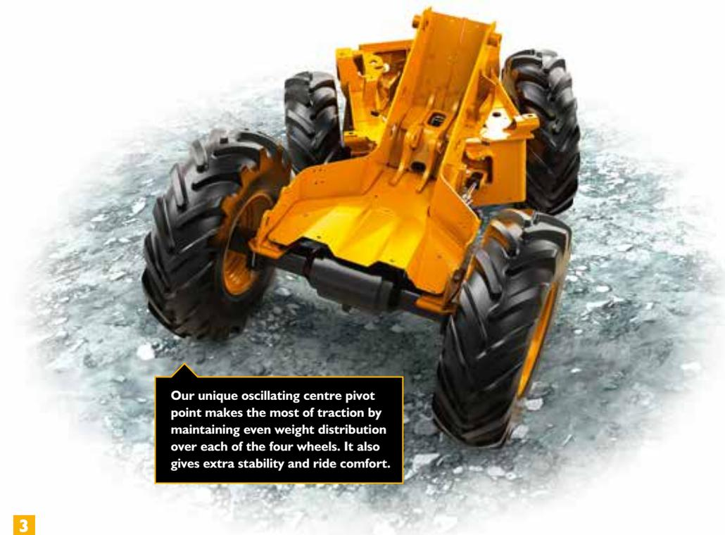
Our unique oscillating centre pivot point makes the most of traction by maintaining even weight distribution over each of the four wheels. It also gives extra stability and ride comfort.
