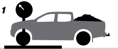
1 Load placed over the front half of the vehicle determines front spring selection Ensure total weight does not exceed manufacturers axle load limit
