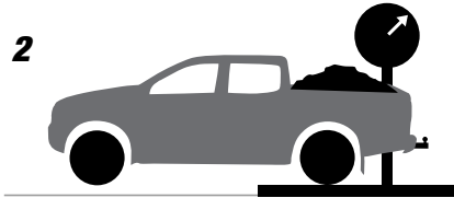
2 Load placed over the rear half of the vehicle determines rear spring selection Ensure total weight does not exceed manufacturers axle load limit
