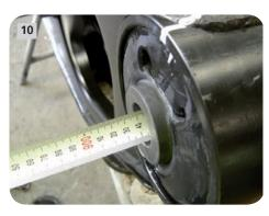
IMPORTANT: After the pivot bush replacement, ensure that all components are assembled and installed correctly. All bolts must be on the recommended torque settings. Ensure that the correct air pressure is in the air suspension system and check the ride height. Check the axle alignment and tighten the pivot bolt as per SAF-HOLLAND recommendations.
