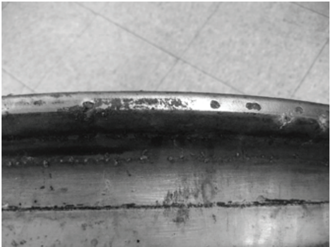
Picture 13-37 Acceptable wear and pitting
