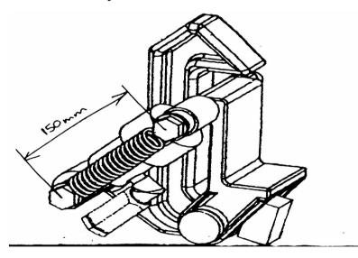
Failure to set this on installation may cause the cylinder to fail prematurely.
