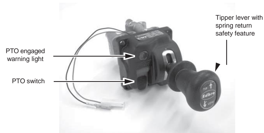
Fig. a. Combined PTO & tipper air controls
