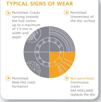
Current damage pattern standard in accordance with the SAF-HOLLAND maintenance
