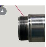
Wipe any dust or residue off of the damaged thread and moisten it with a suitable cleaner.
