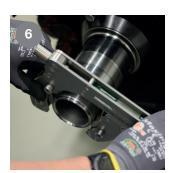
Using rotating movements, roll the damaged thread over the entire thread area in several passes. Note: Retighten the clamp screw if necessary!
