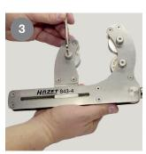
Fasten the rollers onto the thread rolling device.
