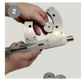
If necessary, insert the appropriate rollers into the thread rolling die. CAUTION: Pay attention to righthand and left-hand threads!
