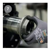
Check whether the axle nut can be screwed onto the thread <u>by hand</u>. It may be necessary to repeat the re-rolling process.
