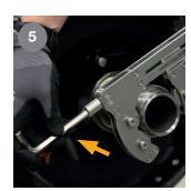
Place the thread rolling die on top of the thread being repaired and tighten it using the clamp screw. The rollers have to fit correctly into the still intact thread flanks!
