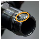
Check the damaged thread using the boundary sample (Chapter 2. Boundary sample, Page 4).
