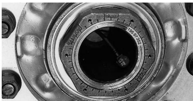
Identification of axles without type plate Production No. of axle on right of axle tube as seen in direction of forward travel.
