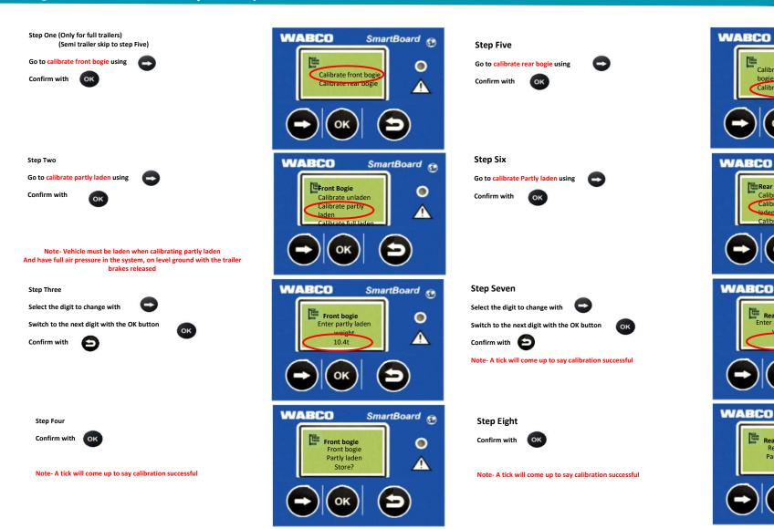
Note- try calibrating using the partially laden option first, if this does not work enter the weights into the full calibration option. This is due to the loads usually not up to GVM of the trailer
