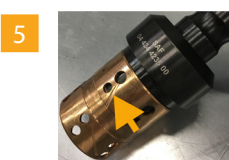
Using Assembly mandrel# 2 install new bearing bushes Pay attention to position of lubrication channels marked in yellow.
