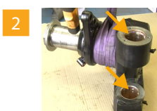
Steering Knuckle with upper and lower bearing bush.
