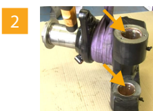
Steering Knuckle with upper and lower bearing bush.
