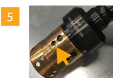
Using Assembly mandrel # 2 install new bearing bushes Pay attention to position of lubrication channels marked in yellow.
