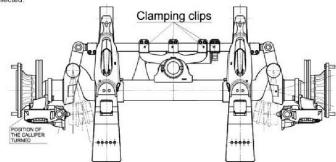
Measuring the axle geometry: Deviations in the distances  $AC - BD = 0 \pm 3$  mm
