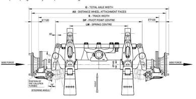
As the side forces decrease, the spring force increases in comparison with the side forces, and forces the tyres and/or steering knuckles back into the straight position. The spiral spring, supported by the damper properties, is also the reason for a sturdy and flutter-free straight drive.
