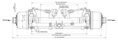
As the side forces decrease, the force in the stabilising cylinder increases in comparison with the side forces and forces the tyres and/ or steering knuckles back into the straight position. The steering damper supports a sturdy and flutter-free drive.
