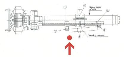
The red dot must be facing to the ground after installation!
