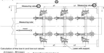
$\frac{AI(IIIII) - BI(IIIIII)}{A(m)} = C \qquad \begin{array}{c} C \text{ (positive value) = toe-in} \\ C \text{ (negative value) = toe-out} \\ \end{array}$ Observe the operating and setting instructions of the measuring system manufacturer
