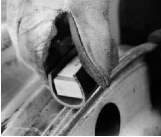
Photo 2. A rubber sharpness gauge constructed from a section of tyre side wall or a suitable piece of rubber attached to a block of wood.
