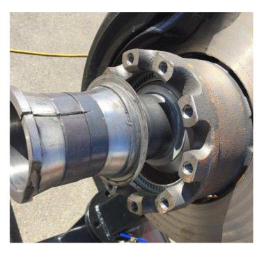
Clean and prepare spindle for installation of replacement hub
