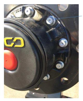
Rotor bolts 15mm socket
