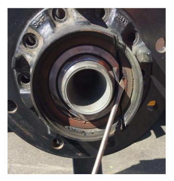
Using a screwdriver break the plastic bearing cage and remove all the rollers from the outer bearing
