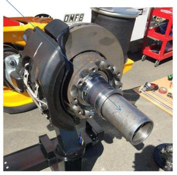
Using a 4" cutting disc, cut a slot along the top of the bearing race
